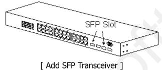
1. Plug in the SFP Transceiver to SFP slot directly.
