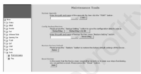
**System Upgrade** : This function will upgrade the system operation software from the web management PC.
