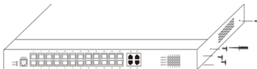
Figure 3-1 Fixing the machine box of the switch
