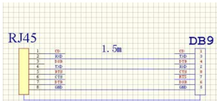
Figure 3-5 Cable connection at the console port
