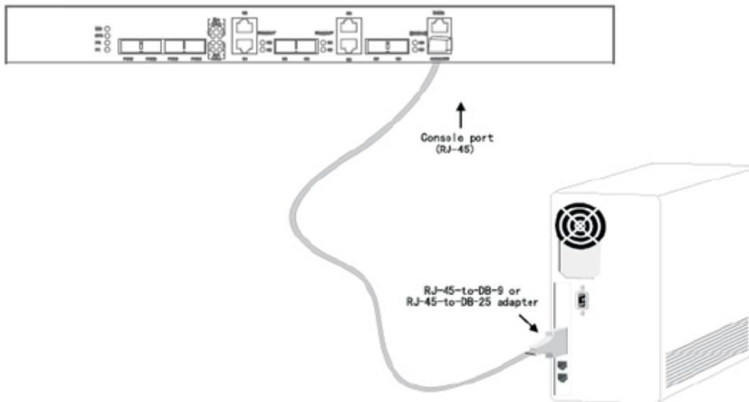
Figure 3-4 Connecting the console port of BDCOM P3310B EPON and the computer
