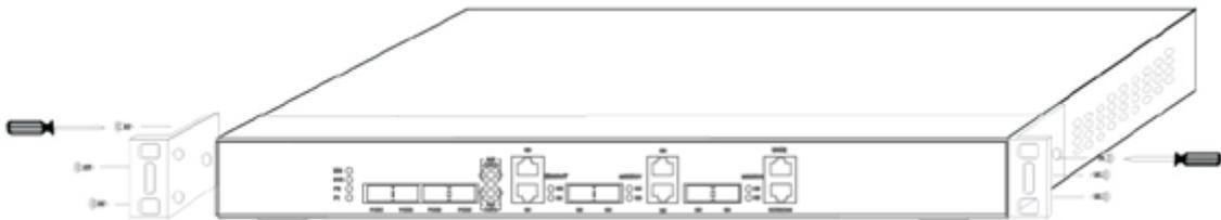
Figure 3-1 Fixing the machine box of BDCOM P3310B EPON to the cabinet
